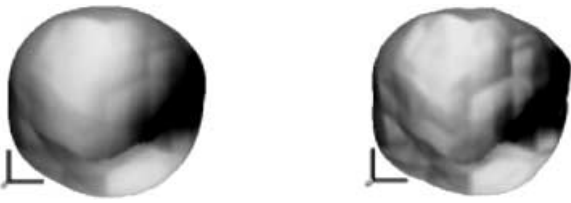
Fig. 20: Shape of smooth (left) and rough (right) particles.
