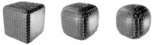
Fig. 2: Form of rounded cubes used for computation e = n = 0.2; 0.5; 0.7 (left to right). In the examples the dimensions are a = b = c = 0.3 \mu\text{m} and the numbers of triangular patches are 1448, 1448, 1400.
