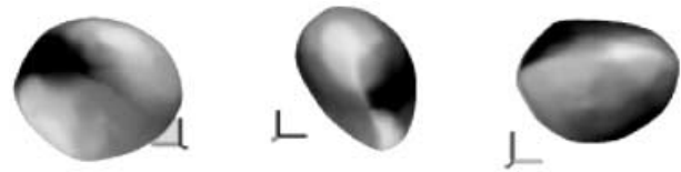
Fig. 18: Three views of “realistically” shaped particle.
