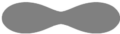
Fig. 7. Cross section of the investigated Cassini shape. The Cassini parameters are a = 1.1 \mu\text{m} , b = 1.125 \mu\text{m} , c = 0.66 . The resulting diameter is d = 3.78 \mu\text{m} and the aspect ratio is 4:1.
